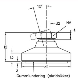
d1 = 50 d2 = M12 l2 = 27.5 l3 = 7.0 NV = 17.0 Static load (N) = 10000 t min = 11.5
